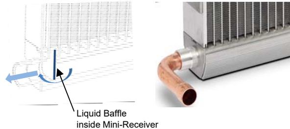
Proper coil orientation and Refrigerant INLET and OUTLET is required. Orienting the coil upside down will result in loss of capacity and high condensing temperatures.
